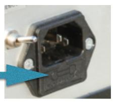
WE ABSOLUTELY DO NOT ALLOW changing the fuses for any larger size than 2A or installing the "audiophile silver bolts" in place of the fuse. Fuses are there mainly to SAVE YOUR LIFE. And we mean that. You can experiment with audiophile grade fuses but not DEAD BOLTS please.
